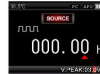
Figure 25 Frequency output
