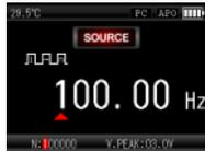
Figure 27 Pulse output
