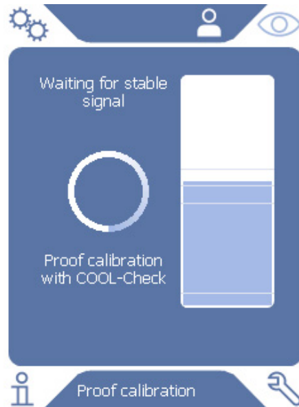
Fig. 12: Display when calibrating internally
