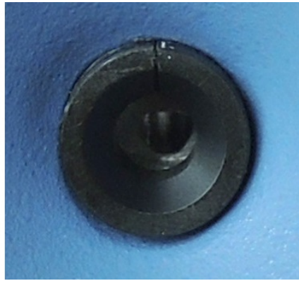
Fig. 10: Insert centering ring
