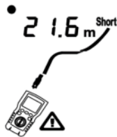
Figure 6.16 Short on Coaxial Cabling
