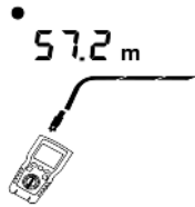
Figure 6.15 Open on Coaxial Cabling
